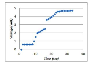
Fig. 7. Variation of LVDT signal with input movement at time.
