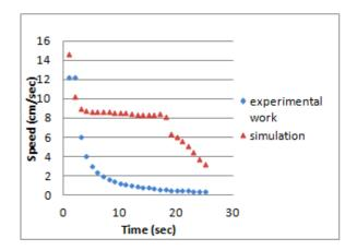
Fig. 13. Comparison in speed between experimental and simulation results.
