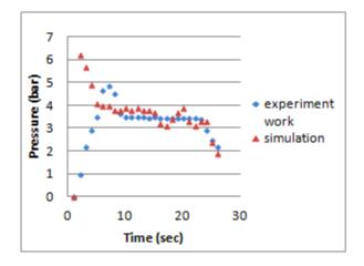
Fig. 15. Comparison in pressure between experimental and simulation results.
