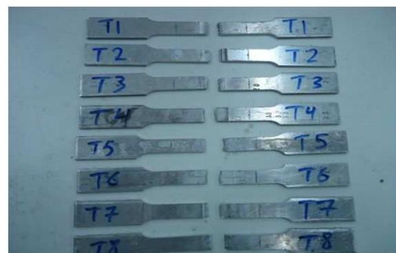
Fig. 7b. Tensile test specimens after testing.
