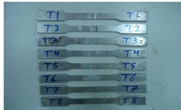
Fig. 7a. Tensile test specimens before testing.
