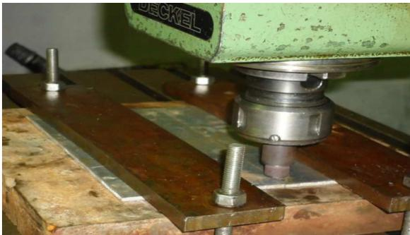
Fig. 3. Welding backing plate and fixtures in use for FSW.
