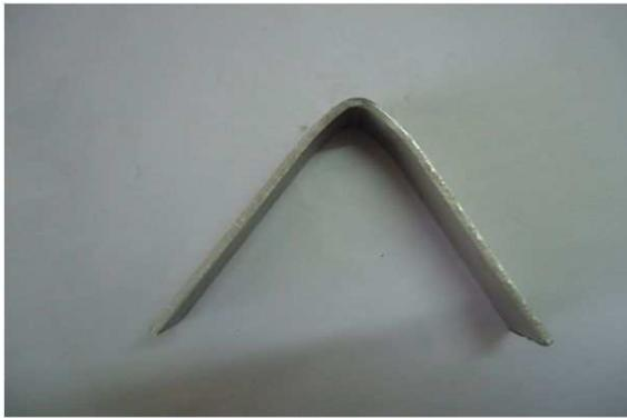
Fig. 8. Bending test specimen after testing.
