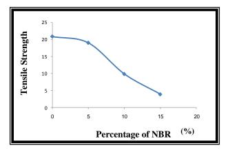
Fig. 3. Tensile strength of Nitrile Rubber (NBR) modified resin (UPE).
