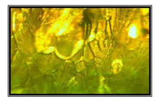
Fig. 6. Optical micrograph of fracture surface for pure(UPE) after tensile test.
