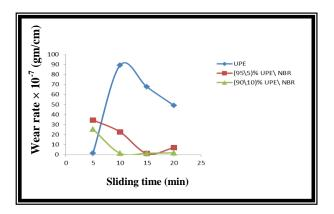
Fig. 5. Variation of wear rate with sliding time for Nitrile Rubber (NBR) modified resin (UPE).
