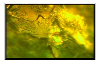
Fig. 7. Optical micrograph of fracture surface for Nitrile Rubber (5%NBR) modified resin (UPE) after tensile test.
