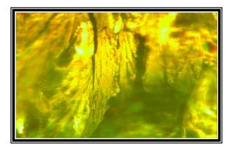
Fig. 8. Optical micrograph of fracture surface for Nitrile Rubber (10%NBR) modified resin (UPE).
