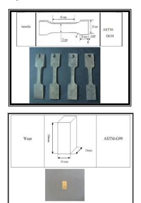
Fig. 1. Samples dimensions and photographs of tensile and wear samples.
