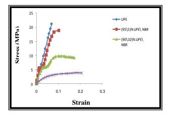
Fig. 2. Stress-Strain curve for UPE and its polymer blends.
