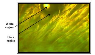
Fig. 9. Optical micrograph of fracture surface for Nitrile Rubber (15%NBR) modified resin (UPE).
