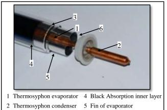
Fig. 3. Evacuated Tubular collector with description notes.
