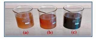
Fig. 4. The stability condition of nano lubricants after 60 days (a) TiO<sub>2</sub>/oil (b) base oil, and (c) CuO NPs.
