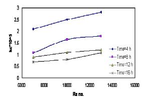
Fig.2. Variation of Mass Transfer Coefficient with Reynolds Number at Different Time Intervals.
