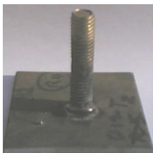
Stud diameter: 12 mm Run: 4, Trial: 2 Monitored Current Peak Value: 652 A
