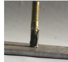
Stud diameter: 10 mm Run: 6, Trial: 1 Monitored Current Peak Value: 477 A
