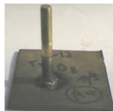
Stud diameter: 8 mm Run: 4, Trial: 2 Monitored Current Peak Value: 320 A
