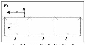
Fig. 2. Location of the Braking Force F<sub>b</sub>
