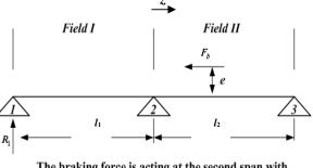
The braking force is acting at the second span with Beam of two fields (span)
