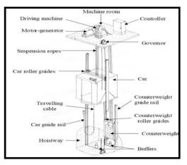
Fig. 1. Components of Elevators
