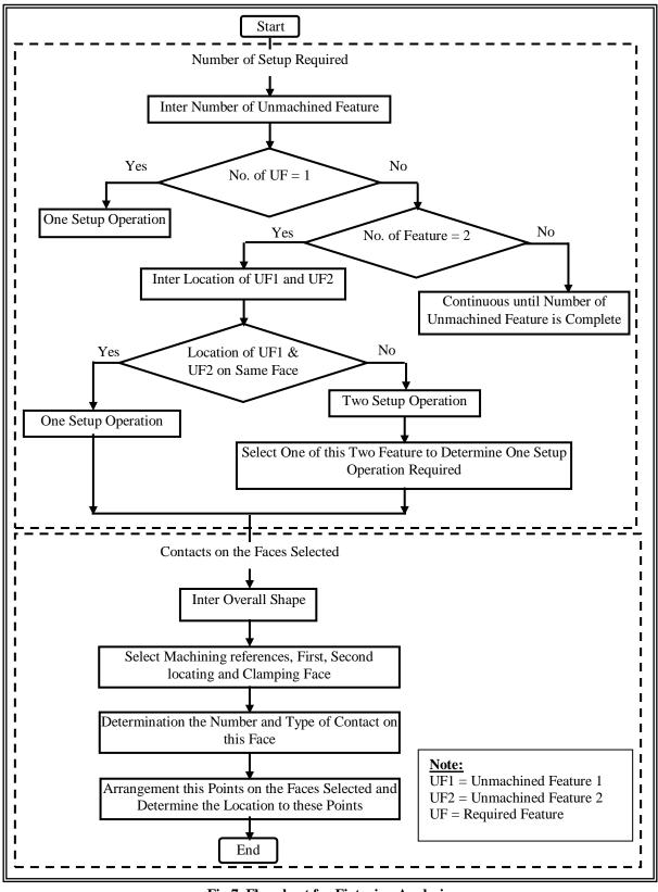
Fig.7. Flowchart for Fixturing Analysis.
