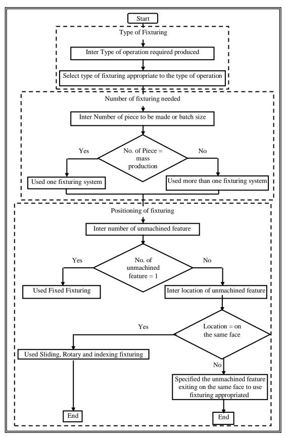
Fig. 5. Algorithm for Fixturing Plan.
