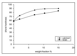
Fig.4. The Relation Between Shore Hardness of LDPE with Weight Fraction of Both Grain and Calcined kaolin Filler.
