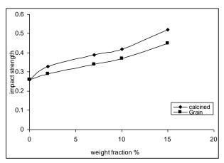
Fig.6. The Relation Between Impact Strength of LDPE With Weight Fraction of Both Grain and Calcined Kaolin Filler.
