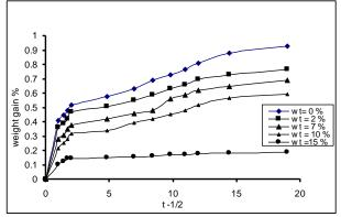
Fig.8. Shows the Relation Between the Weight Gains % of LDPE/Calcined Kaolin With the Square Root of Time.
