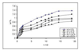
Fig.7. Shows the Relation Between the Weight Gains %of LDPE/ grain Kaolin With the Square Root of Time.
