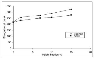
Fig.3. The Relation Between Elongation at Break of LDPE With Weight Fraction of Grain and Calcined kaolin Filler.
