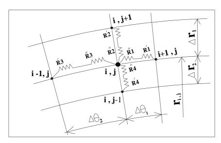
Fig.(3). Thermal Resistances Around Node i,j
