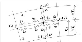
Fig.(a1): Thermal Resistances Around Node (i,j) Located at interfacial line
