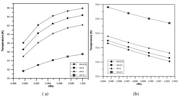
Fig.(7): Aspect Ratio Effect on Temperature Distribution Along Line H-H .
