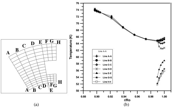
Fig.(5):a). Selected Lines Through Thrust Cell. b). Radial Temperature Distribution of Thrust Chamber Cell For (AR=8.25 )
