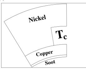
Fig.(1). a).Rocket Thrust Chamber Nozzle. b )Cross Section Through AA. c). Layers of the Wall
