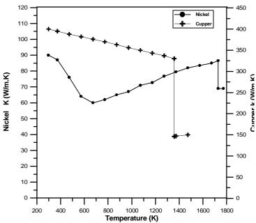
Fig. (4): Thermal Conductivity of Cupper and Nickel [Kacynski]
