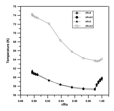
Fig.(6): Aspect Ratio Effect on Temperature Distribution Along Line A-A( Only Convection Boundary Condition)
