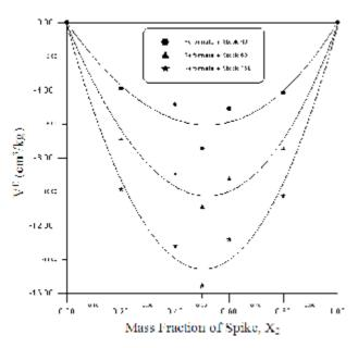
Fig.10. Excess Volume VE for Binary Mixtures of Stock Oil/ Reformate at 40 °C.
