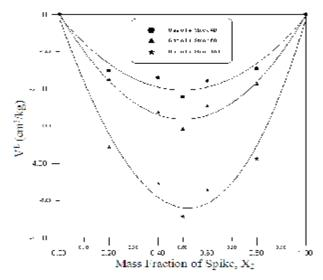
Fig.9. Excess Volume VE for Binary Mixtures of Stock Oil/ Gas Oil at 40 °C.
