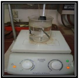
Fig. 2. Carbon Steel Specimen Immersed in Mixture of Corrosion Inhibitor on Hot Plate and Stirrer at Meduim Velocity.
