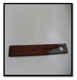
Fig. 7.Uniform Corrosion on Carbon Steel Specimen.
