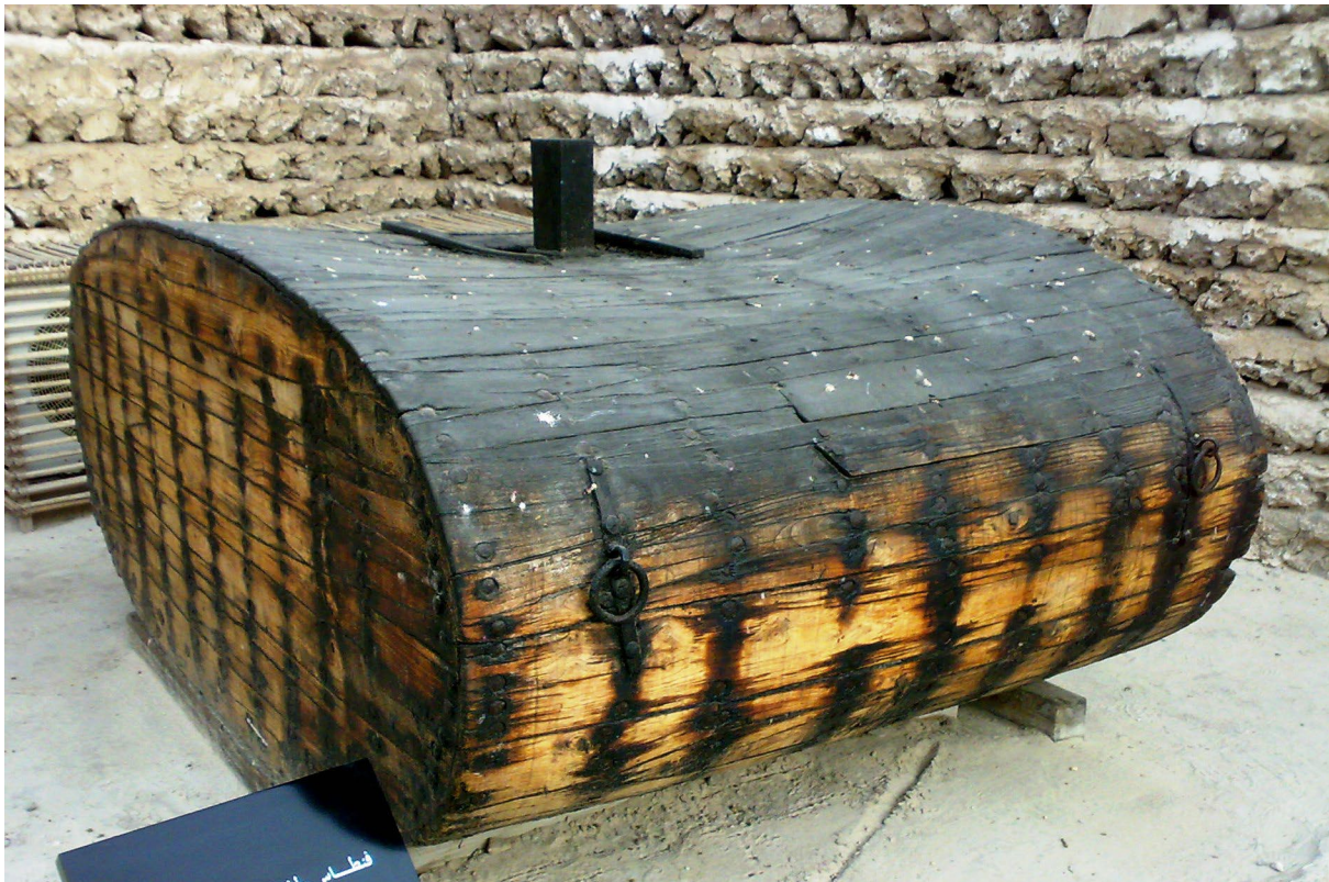
Figure 2: A traditional Arabian ship’s tank ( fintās ), wood and iron, capacity unknown. Probably nineteenth century, Dubai Museum (Al Fahidi Fort), United Arab Emirates. (Photograph by Bjoertvedt, CC BY-SA)
