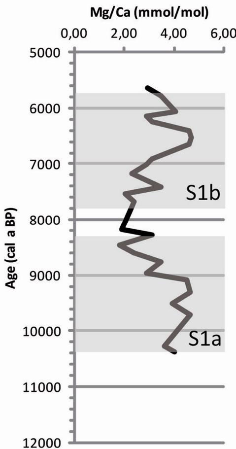
Fig. 3 - Down-core Mg/Ca ratios of *G. ruber* var. *alba* for core ET99M11 across the sapropel S1. The grey areas, representing the extent of the two sub-units of the sapropel S1, are from Vigliotti et al. (2011).
