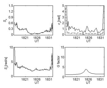
**Fig. 5.** Scintillation indices recorded during the night of 30 October 2003 from the ground station located in Kiruna (for a time interval different than in fig. 4). The solid lines refer to a detrending cut-off frequency of 0.1 Hz, the dashed lines to 0.3 Hz, and the dotted lines to 0.5 Hz. Also shown the geometrical factor G for this satellite link.
