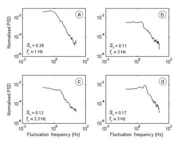
**Fig. 2a-d.** Intensity power spectral densities normalised to the mean received intensity, as measured for different satellite links. This shows that a Fresnel frequency of a few Hz may normally occur at auroral latitudes. The measurements are taken during the night of 30 october 2003 from a) Kokkola, b) Kiruna, c) and d) Lulea.
