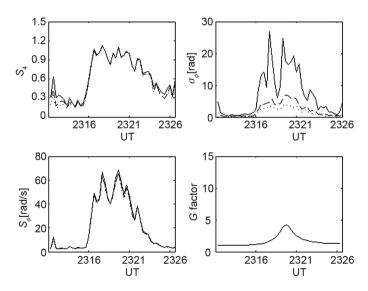
Fig. 4. Scintillation indices recorded during the night of 30 October 2003 from the ground station located in Kiruna. The solid lines refer to a detrending cut-off frequency of  $0.1 \, \text{Hz}$ , the dashed lines to  $0.3 \, \text{Hz}$ , and the dotted lines to  $0.5 \, \text{Hz}$ . Also shown the geometrical factor G for this satellite link.
