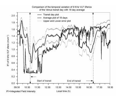
**Fig. 2.** Variation of atmospheric Integrated Field Intensity (IFI) at 9 kHz VLF on the day of Venus transit, 8th June 2004 (continuous line) and average variation of the same parameter around 8th June for 18 days (dotted line) and the dotted grey lines represent standard deviation.
