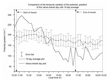
**Fig. 3.** Variation of atmospheric vertical potential gradient on the day of Venus transit, 8th June 2004 (continuous line) and average variation of the same parameter around 8th June for 18 days (dotted line).
