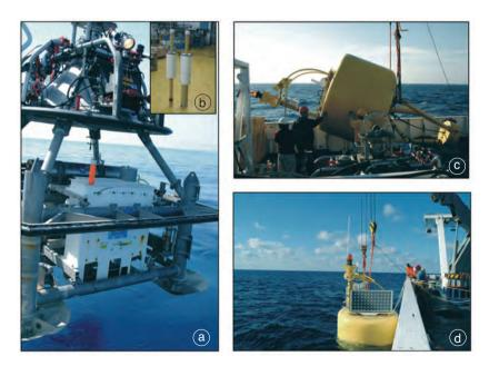
Fig. 5a-d. a) MESSENGERS installed on the Bottom Station (height 1.3 m); b) MESSENGERS Storage and Expendable-type in Brest IFREMER Laboratory; c) surface buoy (weight: 35 kN; volume: 5 m<sup>3</sup>) GEOSTAR-2 version on board R/V Urania; d) surface buoy ORION-GEOSTAR-3 version just deployed.
