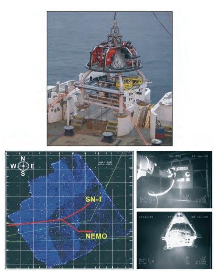
**Fig. 6.** SN-1 and MODUS (*left*) on the deck of the cable-vessel Pertinacia before deployment; the ROV connecting SN-1 Observatory to the cable interface (*top-right*); SN-1 on the seafloor during the cable connecting operations (*bottom-right*). The cable route from Catania harbour to 25-km east in the Ionian Sea is shown in top-left panel.
