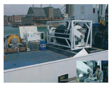
Fig. 4. The GEOSTAR handling system: power unit (*right*), cable spooled on the winch (*left*) and system console (insert).
