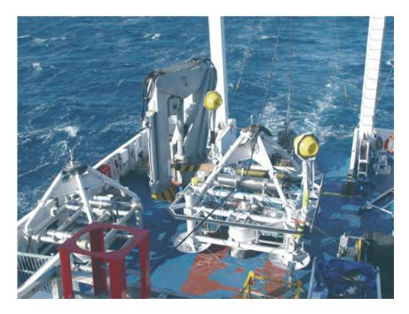
**Fig. 12.** GEOSTAR gateway seafloor observatory (*right*) and ORION Node 3 (*left*) on the deck of the R/V Urania before the deployment at the base of Marsili underwater volcano (ORION-GEOSTAR-3 first mission).
