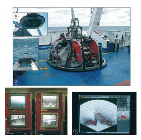
Fig. 3a-e. MODUS, the GEOSTAR deployment/recovery vehicle: a) docking cone and b) pin; c) MODUS on the deck of R/V Urania; d) MODUS on-board console; e) Bottom Station signature displayed on the sonar monitor.
