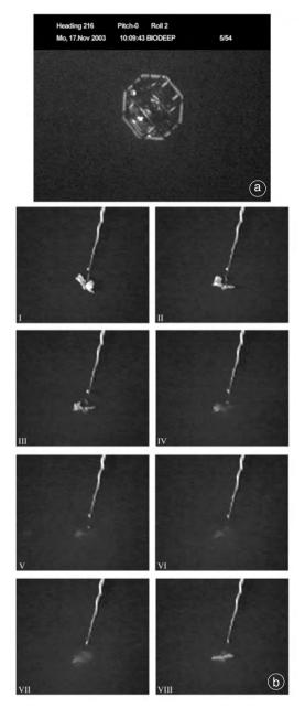
**Fig. 6a,b.** Images of the interface as seen by MO-DUS: a) view from MODUS to the suspended SCI-PACK (10 m mechanical cable) right before entering the Urania Basin; b) sequence of the survey at the interface of L'Atalante (10 m cable): iron ball and flag approaching the interface (I-III), entering the brines (IV), laying below the interface (V-VII) and coming out (VIII).
