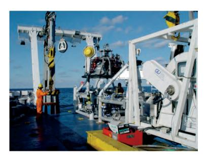
Fig. 1. MODUS and GEOSTAR-stations onboard R/V Urania.
