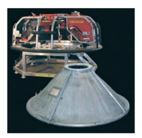
Fig. 2. MODUS with SCISKID (background) and docking cone (foreground).
