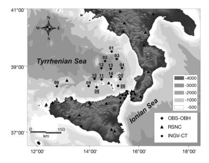
**Fig. 1.** Location of OBS-OBH (diamonds) and land-based seismic stations (triangles and squares) used in the present work. Each ocean bottom station was equipped with an OBH (1 channel), those equipped with an additional 3-component seismic sensor (OBS) are represented by underlined numbers. Station no. 07 is not reported on the map as it was not recovered. The label 00 reports the position of the GEOSTAR multi-parametric observatory, hosting an OBH.
