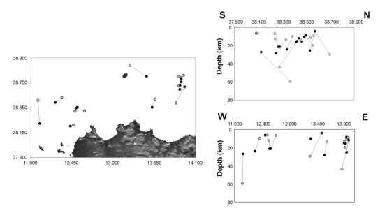
**Fig. 5.** Cluster 2 – Ustica. Grey circles represent the located events using the land-stations; black circles are the integrated locations. Black lines join the two different locations of the same event. On the right, S-N and W-E sections are presented.
