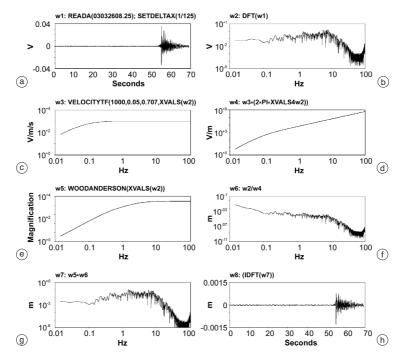
**Fig. 3a-h.** The DaDisp worksheet used to simulate a seismic signal recorded by standard Wood-Anderson seismometer. a) Velocity seismic signal recorded by geophone; b) DFT of velocity seismic signal; c) velocity response curve of geophone; d) displacement response curve of geophone; e) Wood-Anderson response curve; f) velocity spectrum divided by displacement response curve; g) corrected spectrum multiplied by Wood-Anderson simulated seismic signal.
