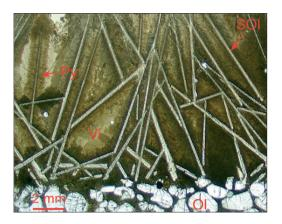
**Fig. 3.** Optical micrograph of remelting product from black sand. Melting condition: 1400°C, 0.45 h in air; Ol – residual olivine phenocrysts; SOL– skeletal olivine
