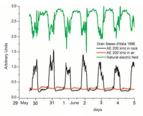
**Fig. 1.** Records in the Gran Sasso area, May 29 through June 5, 1996, showing AE at 200 kHz both inside rock (lower black) and in air (blank signal, lower light grey) and the natural electric field (upper plot) recorded by metal rod inserted into ground for  $\sim 12$  m (in co-operation with INGV) and used as a receiving antenna tuned on the same frequency.
