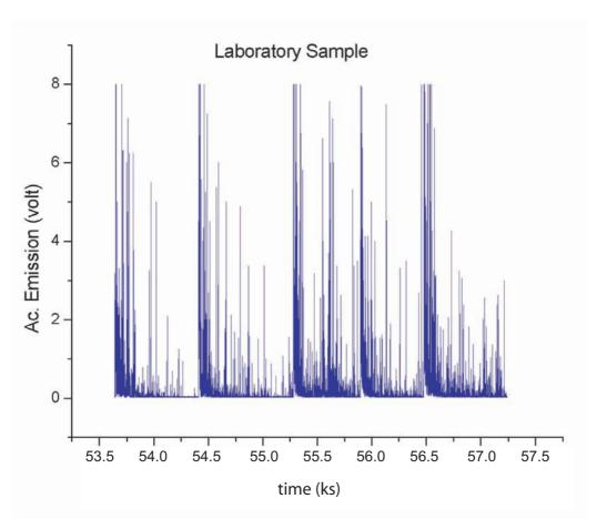
**Fig. 2.** AE bursts recorded during a laboratory experiment. A solid sample composed of a mix of Gran Sasso limestone was compressed and decompressed. The five stronger AE sequences correspond to increased stress. The highest peaks denote amplifier saturation level. The sampling rate is 200 ms. Redrawn after Petri *et al.* (1994) and Vespignani *et al.* (1995).
