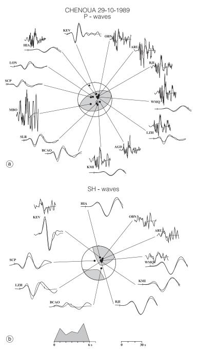
**Fig. 2a,b.** Comparison between observed and synthetic signals for P (a) and SH (b) waves for a single point source inversion (step I). Thick lines: observed signal; thin lines: synthetic signal. Solid and open triangles: P and T axes, respectively.
