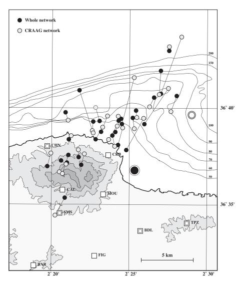
**Fig. 9.** Comparison of the locations calculated with the complete network (CRAAG + IPGS stations) and the locations calculated with the CRAAG stations only. Large open circle: epicenter of the master event; large solid circle: epicenter of the main shock.
