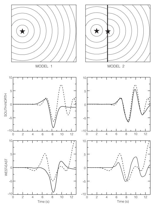
**Fig. 5.** Rupture models from the inversion of the accelerogramm. Continuous line: observed signal; dashed line: synthetic signal.
