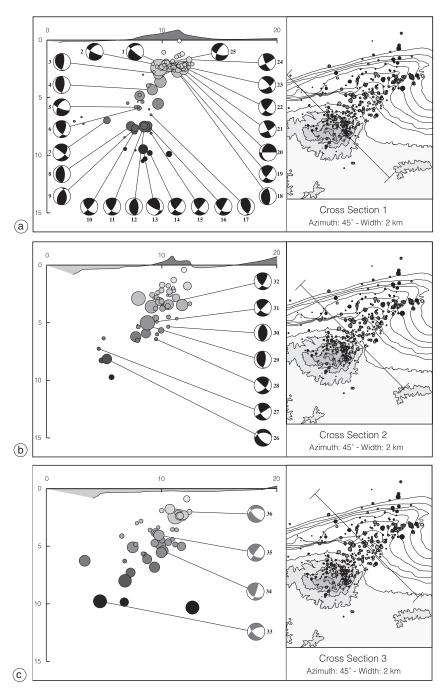
**Fig. 7a-c.** Vertical cross sections through the hypocenters of the aftershocks along the lines shown in the insets. No vertical exaggeration above sea-level, vertical exaggeration under sea-level by a factor 5. The focal mechanisms are shown in the lower hemisphere equal area projection.
