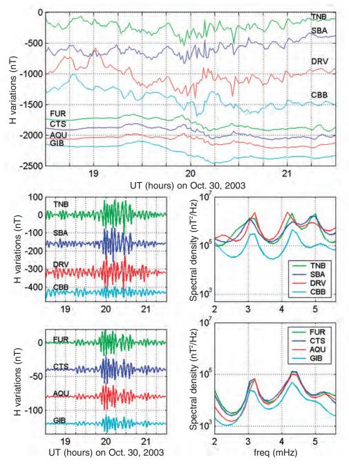
**Fig. 8.** Variations of the H component (unfiltered data, upper plot; 2-5 mHz filtered data, lower left plots) at four high latitude and four low latitude stations (table I) and corresponding power spectra from differenced data (plots on the right).
