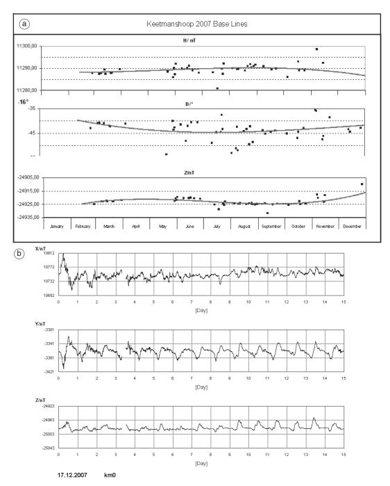
**Fig. 7a,b.** Expamples for data from KMH observatory. a) Measured (black dots) and adopted (grey line) base lines for 2007. b) One minute values of the north (X), east (Y) and vertical (Z) component for the time interval December 17 to 31, 2007.
