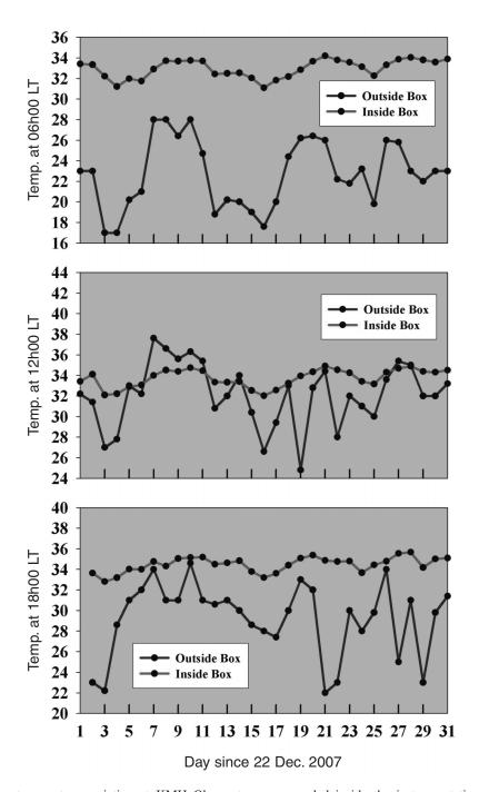
**Fig. 6.** The temperature variation at KMH Observatory as recorded inside the instrumentation box (grey curves) as well as measured outside by the Meteorological Office at the Keetmanshoop Airport at different times of the day (06h00,12h00, and18h00LT). Data shown are from 23 December 2007 till 22 January 2008.
