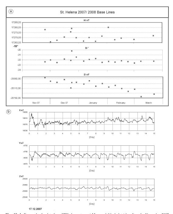
**Fig. 10a,b.** Expamples for data from STH observatory. a) Measured (black dots) baselines for November 2007 to January 2008. The scatter of the first measurements will be reduced as the observer gains experience. b) One minute values of the north (X), east (Y) and vertical (Z) component for the time interval December 17 to 31, 2007.
