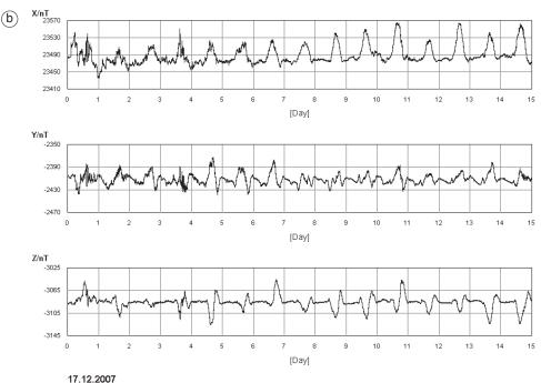
**Fig. 4a,b.** Expamples for data from VRE observatory. a) Measured (black dots) and adopted (grey line) baselines for 2007. The moderate variation is due to seasonal temperature changes in the variometer hut. b) One minute values of the north (X), east (Y) and vertical (Z) component for the time interval December 17 to 31, 2007.
