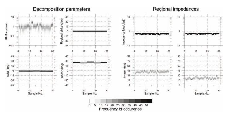
**Figure 3.** *MT* decomposition parameters form the stochastic sampling applied to five groups of six realizations the impedance tensor derived from (17). For each group, the twist and shear parameters are considered constant. The regional strike is assumed to be the same for all data. For details on the figure structure, see caption to Figure 2.
