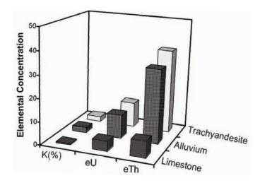
Figure 3. Elemental concentrations for the three types of soil.
