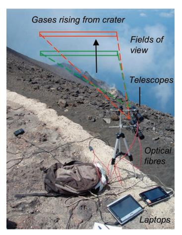
**Figure 3.** Configuration of the wide-angle field-of-view DOAS approach to determine high-time-resolution volcanic SO<sub>2</sub> fluxes, as applied to the rising plume from Stromboli volcano. The orientation of the telescopes, and their quasi-rectangular fields of view are shown, in addition to the fiber connections to the miniature UV spectrometers and the controlling laptops. Note that the spectrometers themselves are concealed within the shade of the backpack.
