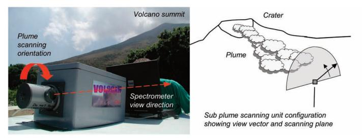
**Figure 2.** Left – Computer-controlled scanning unit situated beneath the plume of Stromboli volcano during SO<sub>2</sub> flux measurements. Right – Schematic representation of the scanning configuration, showing the scan plane inclined nearly perpendicular to the wind direction.
