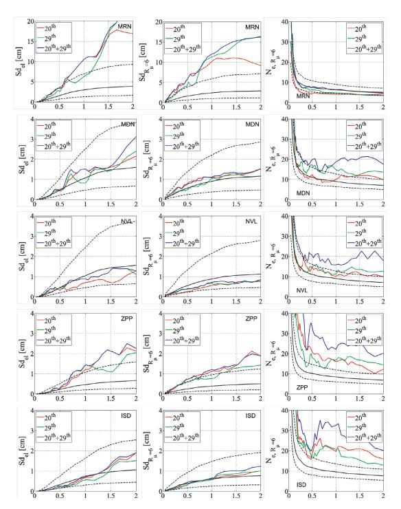
**Figure 8.** Geometric means of the horizontal elastic and inelastic displacements (first two columns), and equivalent number of cycles spectra (third column) evaluated separately for the two events (May 20 and 29, 2012) and for the sequence (20<sup>th</sup> + 29<sup>th</sup>), compared with the GMPEs by De Luca [2011] and De Luca et al. [2012], evaluated for magnitude and distance of the May 20 event. Horizontal axis: always T (s).
