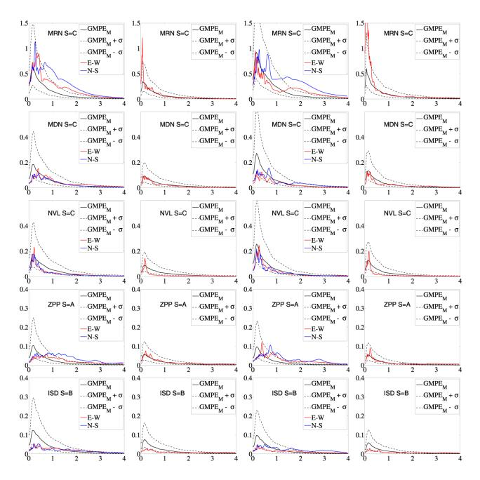
**Figure 5.** Comparison between GMPE-predicted and actual spectra for the May 20 (first and second columns from the left) and the May 29 (third and fourth columns from the left), 2012, events. First and third columns refer to horizontal components, while second and fourth column refer to vertical components. Vertical axis: always  $S_a$  (g); Horizontal axis: always T (s).
