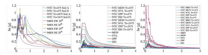
**Figure 6.** Comparison with code spectra for horizontal components of: MRN station (left), of the other four stations (center), and for the vertical components of all of the stations (right). Horizontal axis: always T (s). (Vertical component of MRN might be affected by instrumental error) [see Mirandola Earthquake Working Group 2012].
