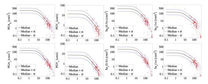
Figure 2. May 20, 2012, event: comparison with the GMPE in terms of PGA, PGV,  $S_a$  (0.3s),  $S_a$  (1.0s), for the geometric mean of the horizontal (h subscript) and for the vertical (v subscript) components of ground motion. Horizontal axis: always  $R_{th}$  (km).
