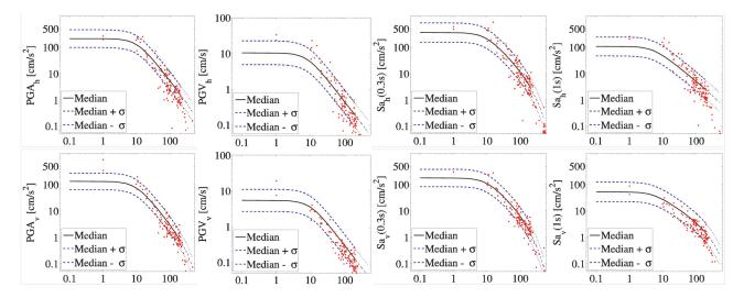
Figure 3. May 29, 2012, event: comparison with the GMPE in terms of PGA, PGV,  $S_a$  (0.3s),  $S_a$  (1.0s), for the geometric mean of the horizontal (h subscript) and for the vertical (v subscript) components of ground motion. Horizontal axis: always  $R_{ib}$  (km).
