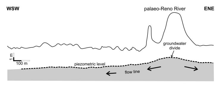
Figure 3. Topographic profile (black line) drawn from a lidar-based DEM, and piezometric level of the unconfined aquifer system (A0), as reconstructed from water-well measurements a few weeks after the seismic event.
