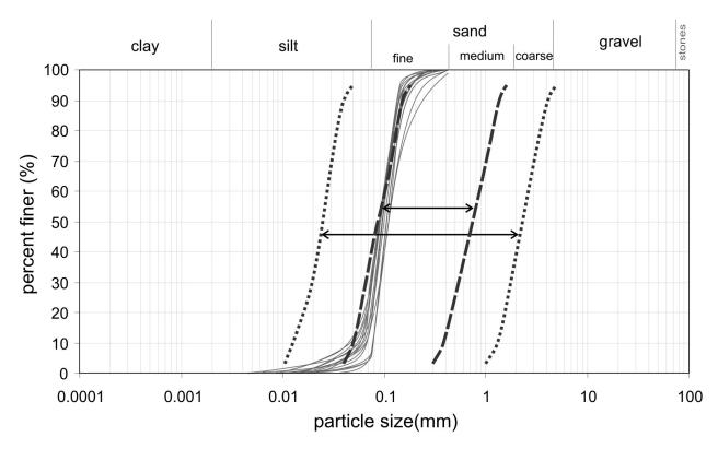
Figure 5. Comparison between the grain-size distribution curves of the collected samples and the boundary curves for liquefiable (dashed lines) and probable liquefiable (dotted lines) soils, as suggested by Tsuchida [1971]. Similar critical curves were proposed by EN 1998-1 [2004] and NTC [2008].
