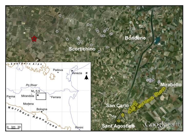
Figure 1. Map of the spatial distribution of the liquefaction-induced surface evidence within the west Ferrara Province from original data (yellow circles) and from the ISPRA [2012] report (white circles). Red star, May 20, 2012, earthquake epicenter. Base map from Google Inc. (2012).
