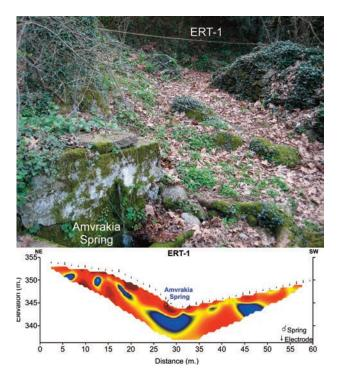
**Figure 5.** The first geoelectrical transverse was established uphill the spring location (above) and the interpreted tomography section, including topographic relief (below) revealed several conductive zones of relatively low resistivity values (ERT-1: 10th iteration, RMS: 2.38%). See Figure 6 for scale values.
