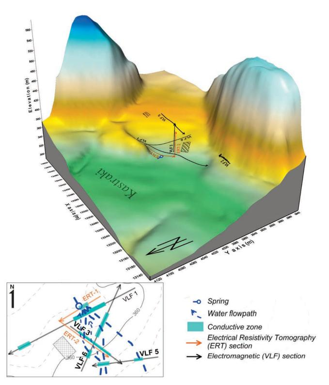
**Figure 4.** A 3-dimensional perspective representation of the study area on which the ERT and the VLF geophysical transverses are indicated. A 2-dimensional map of the same area along with the interpreted conductive zones and the groundwater flow paths is displayed below.
