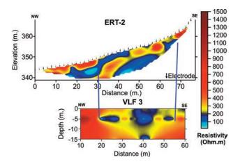
**Figure 6.** Comparison of resistivity sections generated from the inversion of the ERT-2 data values (11th iteration, RMS: 2.74%) and the VLF-3 data inversion with Inv2DVLF. It is clear that both the techniques have produced similar results.
