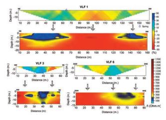
**Figure 7.** The Karous-Hjelt pseudo-sections of the selected profiles VLF 1, VLF 3 and VLF 6 are represented. The respective resistivity section derived from inversion with Inv2DVLF software is also included (Initial resistivity 500 Ohm.m with 20 iterations. RMSVLF 1= 1.16%, RMSVLF 3=1.82%, RMSVLF 6=0.95%). Frequency: 23.4 KHz.
