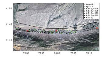
**Figure 4.** Fundamental frequency at single station measurement sites in Naryn. Temporary network (green dots) installed in summer 2013 and array measurement sites (red dots) are also shown. Black lines represent active faults [Arup and Partners Int. Ltd. 2012].
