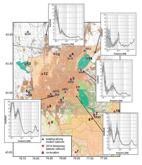
**Figure 8.** Network layout indicating the location of the existing strong motion stations (blue triangles) and weak motion stations (red dots) in the city of Almaty. The embedded images show the noise H/V spectral ratio plus/minus one standard deviation for representative sites in the city. The reddish color shows the actual administrative border of the city. The greenish areas will be incorporated in the future.
