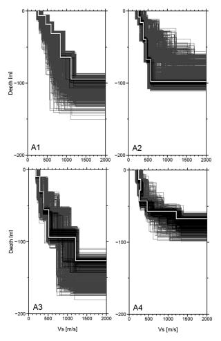
**Figure 6.** Shear-wave velocity profiles for array measurement sites in Dushanbe shown in Figure 5. Thin gray lines show all tested models. The white line represents the minimum cost model and the black lines indicate all models lying inside the minimum cost +10% range.
