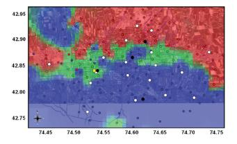
**Figure 2.** Temporary network (white dots) installed in Bishkek in summer 2008, array measurement sites (black dots) and location of the vertical array (yellow rectangle). The color-coded dots represent the location of the single station seismic noise measurement sites. Different colors represent the different clusters or groups.
