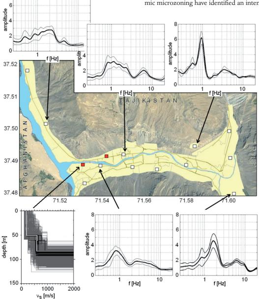
**Figure 7.** Network layout (white dots) and array measurement sites (red dots) in the city of Khorog. Horizontal-to-vertical spectral ratios for earthquakes plus/minus one standard deviation are shown for representative stations. For the western array measurement site the shear-wave velocity profile is shown. Thin gray lines show all tested models. The white line represents the minimum cost model and the black lines indicate all models lying inside the minimum cost +10% range.
