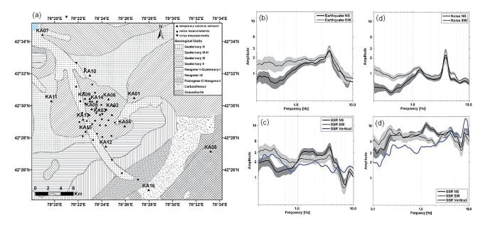
**Figure 3.** (a) Surface soil material for the city of Karakol. Seismic noise measurement sites (black dots) and installation sites of the temporary seismic network (black triangles) are indicated. (b) Horizontal-to-vertical spectral ratio plus/minus one standard deviation for earthquakes for station KA02. (c) H/V spectral ratio for noise at station KA02. (d) SSR for earthquakes for KA02 using KA08 located on bedrock as a reference. (d) SSR for earthquakes for KA07 using KA08 as a reference.
