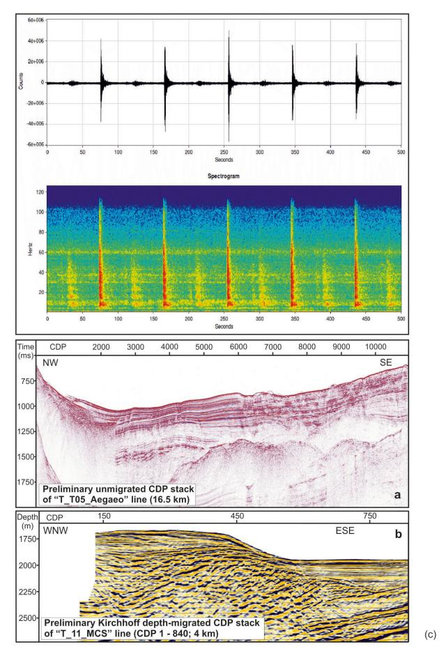
**Figure 2** (continues from previous page). (c) Upper frame: an example of a seismogram and spectrogram of a few shots recorded in an OBS (ocean bottom seismometer) station; bottom frame: preliminary Kirchhoff depth migrated CDP stack of profile T11, shotpoints 400-500.
