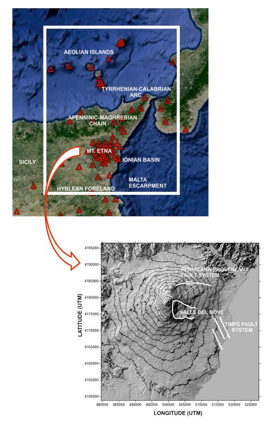
Figure 1. Maps of the area under study in the TOMO-ETNA experiment. Triangles mark the position of the seismic stations of the permanent network of the INGV, Italy. Map was obtained using free Google Earth platform.
