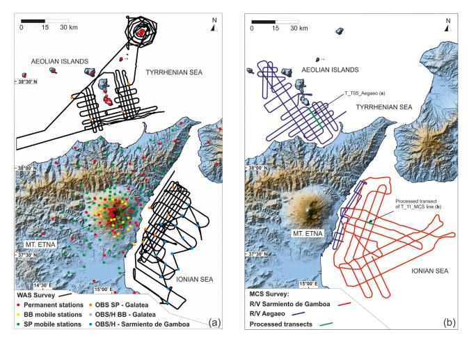
**Figure 2.** Lines of shots: (a) wide angle seismic (WAS) for the "Sarmiento de Gamboa" campaign. Colored dots indicate the position of the seismic stations (see legend in the figure for details); (b) multi-channel seismic (MCS) lines for the "Sarmiento de Gamboa" and "Aegaeo" campaign. (Figure 2 continues on next page.)
