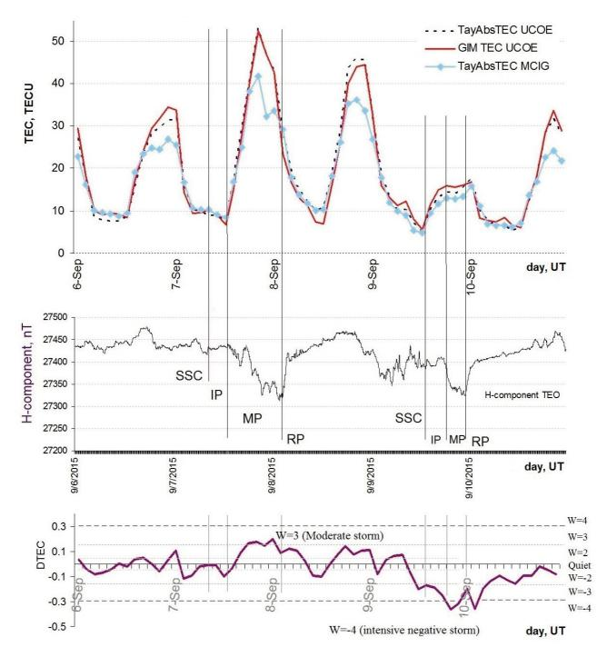
**Figure 2.** TEC by GIM for UCOE station and TEC by TayAbsTEC for UCOE and MCIG stations during September 6-10, 2015 (panel a). Variations of H-component of the magnetic field (panel b). DTEC and ionospheric weather W-index (panel c). IP, MP and RP are the initial, main and recovery phase of the storm respectively. SSC is Sudden Storm Commencement.
