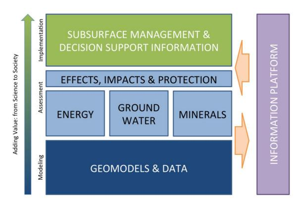
Figure 1: Generic workflow underpinning the presented Geological Service for Europe. In this concept, subsurface management and resource assessments are linked to the consistent 3D geomodels from which they are derived.
