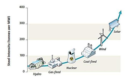
Figure 1: Steel intensity for different power technologies, in tonnes per MW (Wellmer, 2012).
