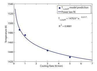
**FIGURE 5.** Plot of the predicted Tcutoff temperatures as a function of cooling rate. Blue circles represent the forecasted values from the data in figure 4 for cooling rates of 0.5, 1, 3 and 5 K/min. the blue solid line represents a power law model fitted to these data describing the  $T_{cutoff}$  lava immobilization threshold as a function of cooling rate. Errors are smaller than symbol size.
