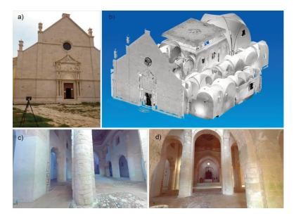
FIGURE 10. Laser scanner Focus 3D MS120 (FARO) (a), mesh visualization of the model (b), RGB visualization of the cloud points (c, d).
