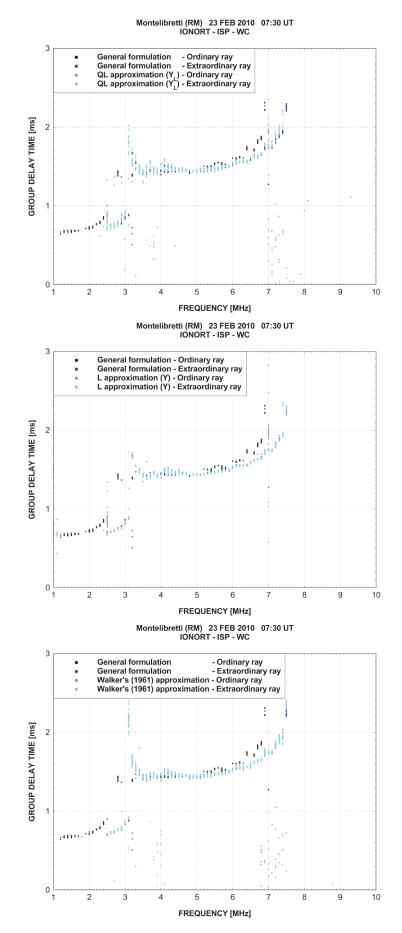
**Figure 5.b.** Corresponding "quasi" vertical ionograms along Rome (TX) – Montelibretti (RX) "short" radio link, synthesized by IONORT-ISP-WC system.
