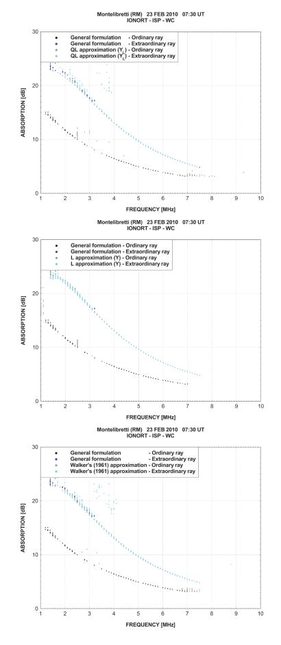
**Figure 5.c.** Corresponding semi-logarithmic plots of the non-deviative absorption L [dB], according to the COMPLEIK model, as a function of the frequency f [MHz].
