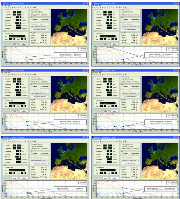
**Figure 3.** Graphical user interface (GUI) of IONORT program. Two simulations are plotted for: (a) a fixed elevation angle of 30°, with a 3 MHz frequency-step procedure from 3 MHz to 30 MHz; and, (b) a fixed frequency of 9 MHz, with a 10° elevation-step procedure from 5° to 85°.
