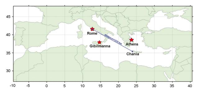
**Figure 2**. Map of the central Mediterranean region considered in this study. Red stars represent the ionospheric stations used as input for the ISP model. In blue, the radio link between Rome and Chania used to test the effectiveness of the IONORT-ISP system.
