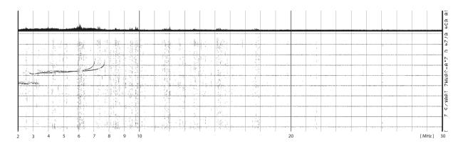
Figure 5.a. Vertical ionogram recorded by AIS-INGV digital ionosonde over Montelibretti (RM) station on 23 February 2010 at 07:30 UT.
