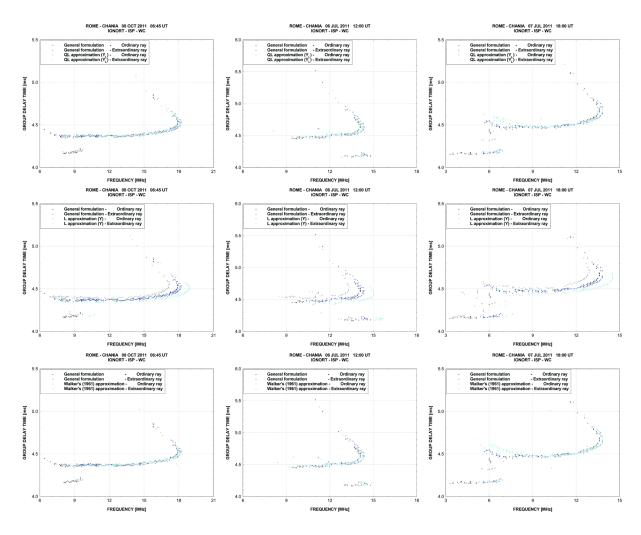
Figure 4.b. Corresponding oblique ionograms synthesized by IONORT-ISP-WC system;.
