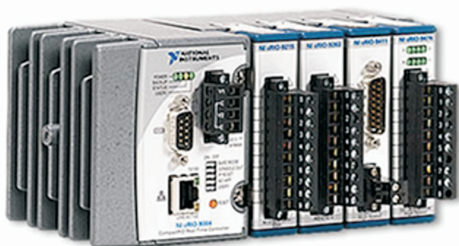
Fig. 8: CompactRio – this programmable automation controller is a low-cost reconfigurable control and acquisition system designed for applications that require high performance and reliability. The system combines an open embedded architecture with small size, extreme ruggedness, and hot-swappable industrial I/O modules. NI CompactRIO is powered by reconfigurable I/O (RIO) FPGA technology. NI CompactRio is compatible with the LabView development system.
