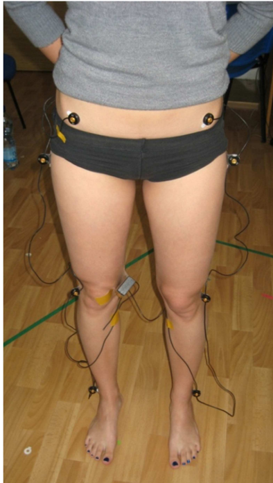
Fig. 1: Location of IR markers and angles measured during the examination
