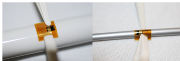
Figure 14: Bending tests with a pen (5 mm radius) and with a ball pen refill (1.5 mm radius).
