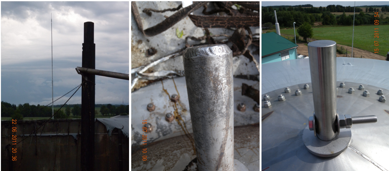
FIGURE 1. A lightning strike to a biogas plant digester, which was supposedly protected by an ESE conductor: damaged masking head after lightning strike (middle), new masking head before lightning strike (right).
