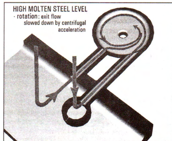
Fig. 5: Horizontal section through the vortex chamber and its inlets, showing both radial and tangential flow at a high level of the metal in the tundish
