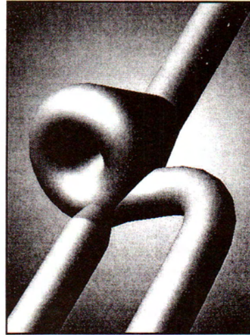
Fig. 11: A version of the tested conical vortex valve, with nozzle contraction in the radial inlet. The obvious advantage of a conical valve is its compactness and small dimensions. This is the shape of the “lost wax” core (in fact an ACIS model) – a “negative” of the valve cavities.
