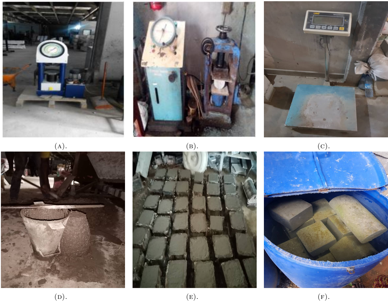
FIGURE 1. Laboratory Equipment and Experimental Activities (a, b) Avery Dension Universal Testing Machine (c) Material Measurement using Weighing Machine (d) Slump Test (e) Casting of Concrete Cubes (f) Concrete Cubes Immersed in Potable Water Curing.
