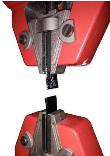
FIGURE 9. Separation of the adhesive joint of the TPU material.
