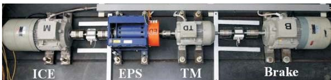
Fig. 3: Electric machines of the laboratory working stand
