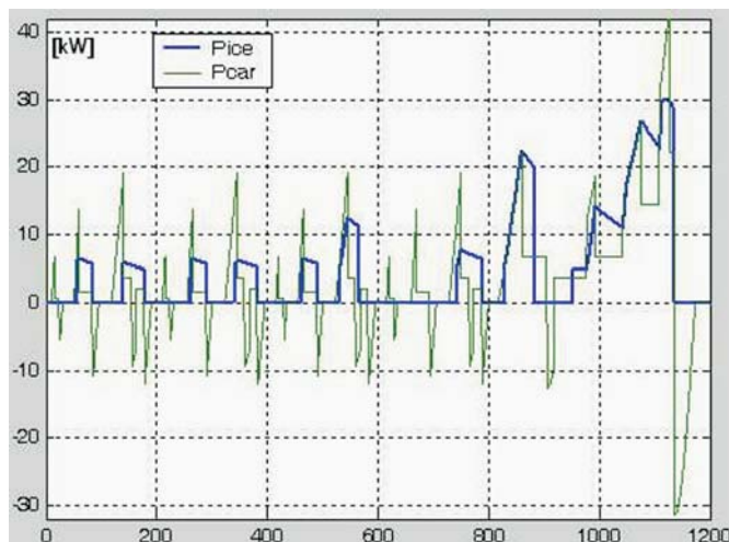
Fig. 5: P_{car} and power produced on the drive shaft of the ICE
