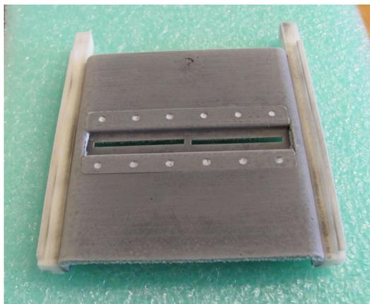
**Figure 2:** The narrow occulting slot that can be moved just in front of the SALTICAM CCDs to allow for high time resolution (down to  $\sim 80$  ms) photometry.
