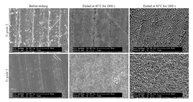
FIGURE 3. SEM images of grade 2 and grade 5 titanium discs before etching and after etching in HCl at  $40^{\circ}$ C and  $60^{\circ}$ C for 1800 seconds.
