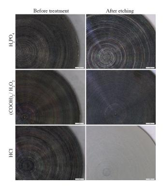
FIGURE 1. Stereo microscopic images of titanium discs before and after etching in  $H_3PO_4$ , in the compound of (COOH)<sub>2</sub> × 2H<sub>2</sub>O and H<sub>2</sub>O<sub>2</sub> and in 30% HCl.
