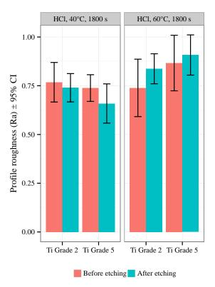
FIGURE 2. Mean profile roughness values and their 95% CIs for Ti grade 2 and Ti grade 5 discs before and after etching in 30% HCl at 40°C for 1800 seconds and at 60°C for the same duration.
